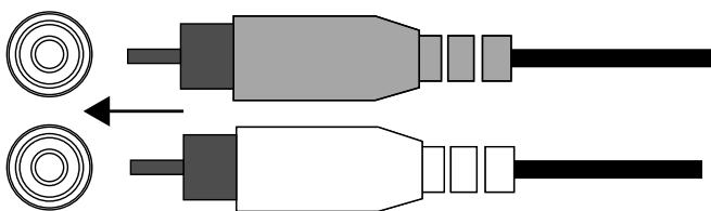
If your car audio system's head unit does not have **line-level outputs**, use the supplied bare wire-to-RCA adapters to connect the Kappa amplifier's inputs to either the front or the rear speaker outputs of your car audio system's head unit (splice crimps not included).
